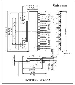
Note) The package of this product will be changed to lead-free type (HZIP016-P-0665D). See the new package dimensions section later of this datasheet.
