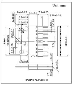
Note) The package of this product will be changed to lead-free type (HSIP009-P-0000E). See the new package dimensions section later of this datasheet.
