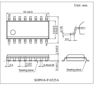
Note) The package of this product will be changed to lead-free type (SOP016-P-0225E). See the new package dimensions section later of this datasheet.
