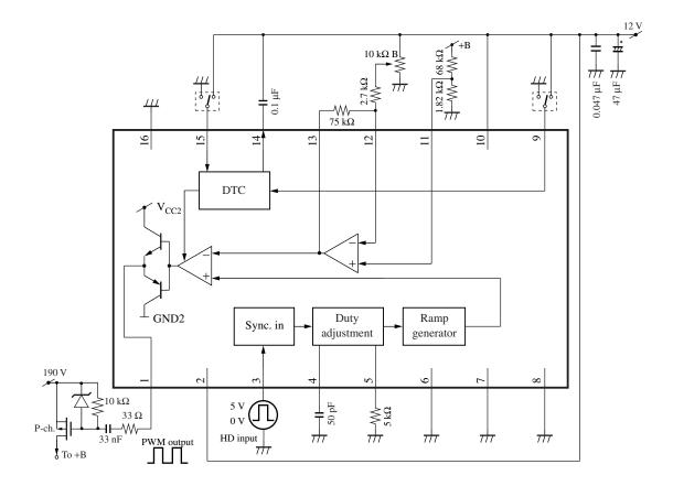
Note) When both of the pin 4 and the pin 5 are open, minimum pulse width of PWM output is 2.0 µs.
