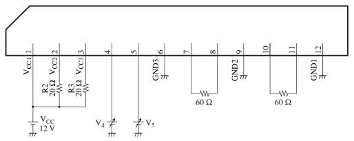
If pin 3 ( $V_{CC3}$ ) becomes a voltage of 8 V or less by making resistance value of R3 larger, the upper limit of output voltage for pin 7 and pin 8 is restricted and then the output becomes as shown in figure 1.
