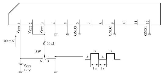
3. The change in output voltage by the  $V_{CC2}$  and  $V_{CC3}$  voltage change
