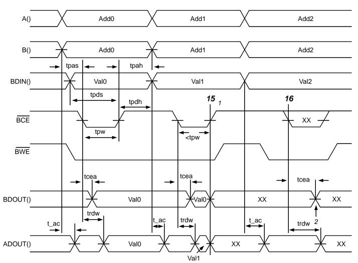
Address setup time to  $\overline{\text{BCE}}$  Address hold time to  $\overline{\text{BCE}}$ Notes: tpas
