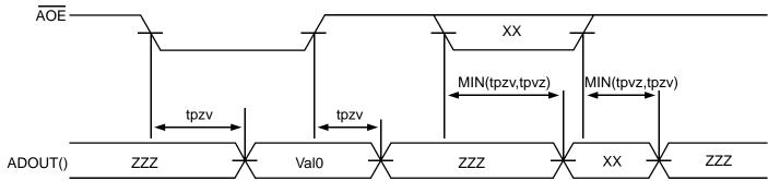
Notes: tpvz : Delay to propagate valid DOUT() to high impedance. tpzv : Delay to propagate high impedance to valid DOUT().
