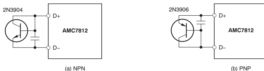
Figure 88. Remote Temperature Sensor Using Transistor
