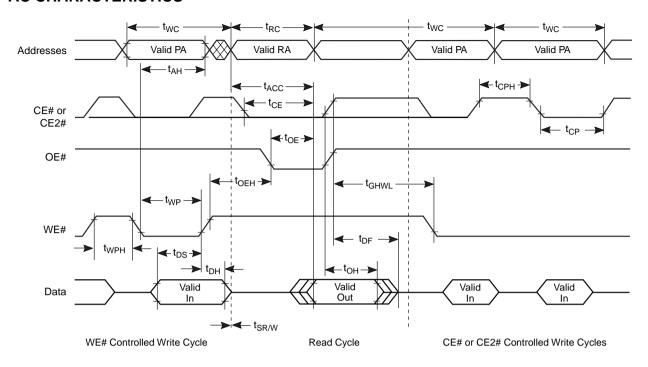
Figure 18. Back-to-back Read/Write Cycle Timings
