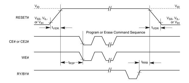
Figure 22. Temporary Sector Unprotect Timing Diagram
