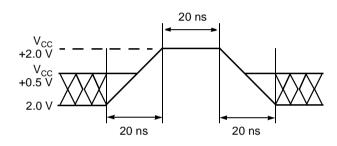
Figure 8. Maximum Positive Overshoot Waveform
