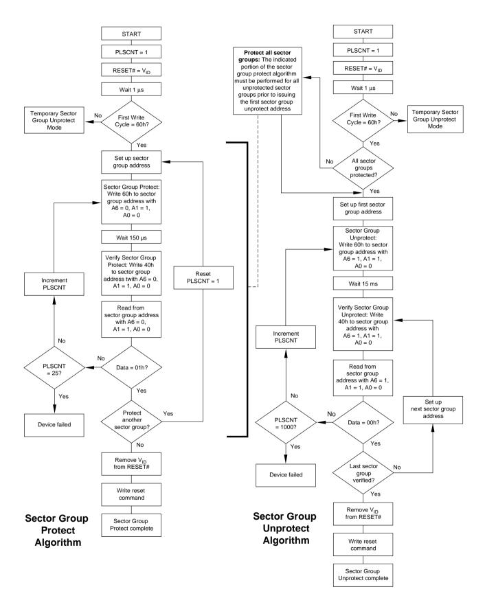
Figure 2. In-System Sector Protect/Unprotect Algorithms
