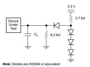
Figure 11. Test Setup
