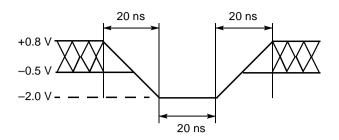
Figure 7. Maximum Negative Overshoot Waveform
