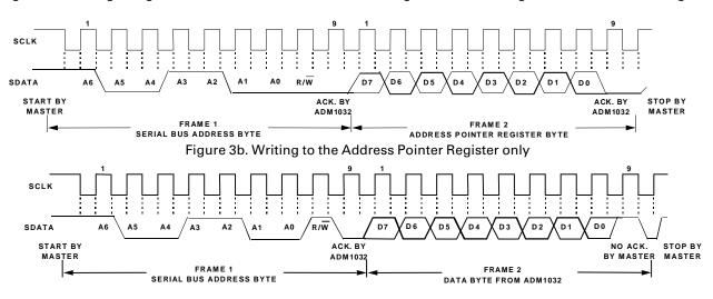
Figure 3c. Reading Data from a Previously Selected Register
