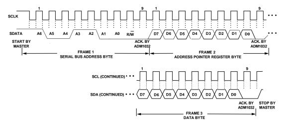
Figure 3a. Writing a Register Address to the Address Pointer Register, then Writing Data to the Selected Register
