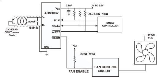
Figure 14. Typical ADM1032 Application Circuit
