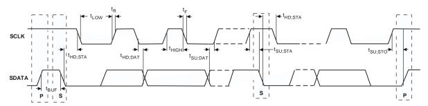
Figure 1. Diagram for Serial Bus Timing
