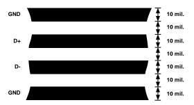
Figure 5. Arrangement of Signal Tracks
