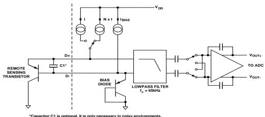
\*Capacitor C1 is optional. It is only necessary in noisy environments. C1= 2.2nF typical, 3nF max
