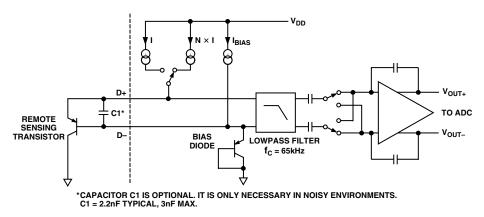
Figure 12. Input Signal Conditioning
