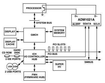
Figure 19. Typical System Using ADM1021A
