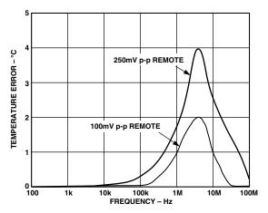
Figure 3. Temperature Error vs. Power Supply Noise Frequency
