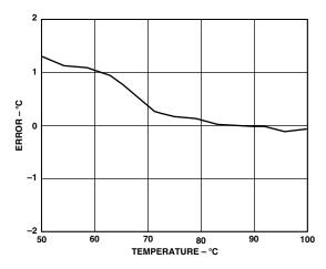
*Figure 5. Temperature Error of ADM1021A vs. Pentium III Temperature*
