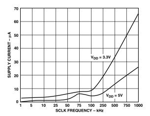
Figure 7. Standby Supply Current vs. Clock Frequency
