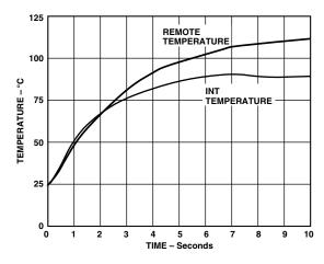
Figure 11. Response to Thermal Shock
