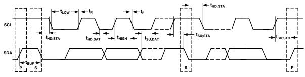
Figure 1. Diagram for Serial Bus Timing
