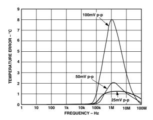
Figure 4. Temperature Error vs. Common-Mode Noise Frequency
