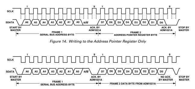
Figure 15. Reading Data from a Previously Selected Register
