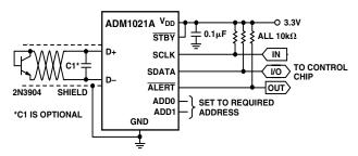
Figure 18. Typical ADM1021A Application Circuit
