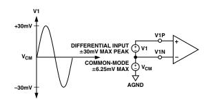
Figure 5. Maximum Signal Levels, Channel V1
