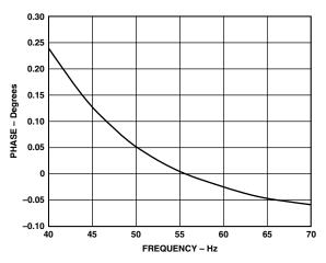
Figure 12. Phase Error between Channels (40 Hz to 70 Hz)
