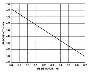
Figure 15. Effect of RCKLIN on Internal Oscillator Frequency (OSC)
