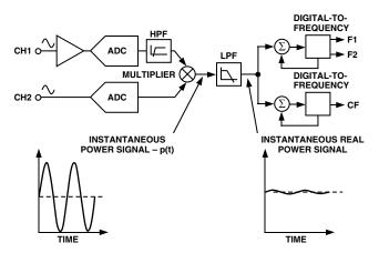
Figure 3. Signal Processing Block Diagram
