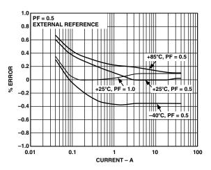
TPC 4. Error as a % of Reading over Temperature with External Reference (PF = 0.5)
