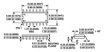
CONTROLLING DIMENSIONS ARE IN MILLIMETERS; INCH DIMENSIONS (IN PARENTHESES) ARE ROUNDED-OFF MILLIMETER EQUIVALENTS FOR REFERENCE ONLY AND ARE NOT APPROPRIATE FOR USE IN DESIGN COMPLIANT TO JEDEC STANDARDS MS-012AC
