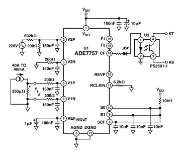
Figure 2. Test Circuit for Performance Curves
