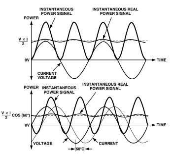
Figure 4. DC Component of Instantaneous Power Signal Conveys Real Power Information PF < 1
