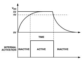
Figure 9. On-Chip Power Supply Monitor
