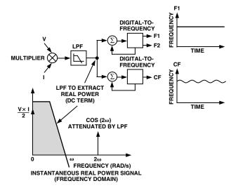
Figure 13. Real Power-to-Frequency Conversion
