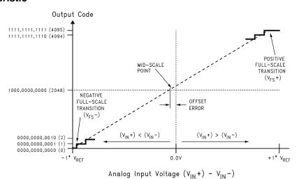
Figure 3. Transfer Characteristic
