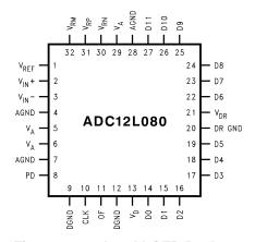
Figure 1. 32-Lead LQFP Package See Package Number NEY0032A
