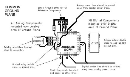
Figure 41. Example of a Suitable Layout
