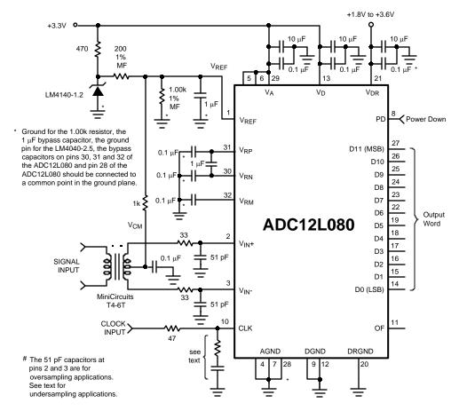
Figure 40. Driving the Signal Inputs with a Transformer
