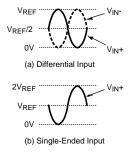
Figure 36. Expected Input Signal Range
