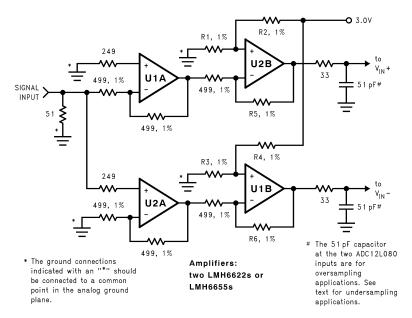
Figure 39. Differential Drive Circuit of Figure 38
