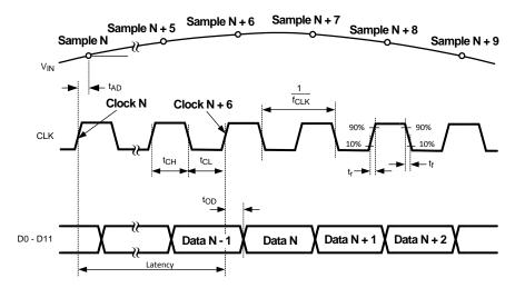
Figure 2. Output Timing
