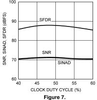
SNR, SINAD, SFDR vs. Clock Duty Cycle, DCS Enabled,  $f_{\text{IN}}\text{=}40~\text{MHz}$
