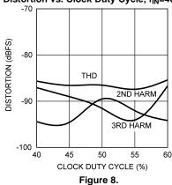
Distortion vs. Clock Duty Cycle, DCS Enabled,  $f_{\text{IN}}$ =40 MHz
