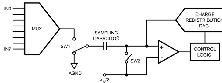
**Figure 5. ADC128S102 in Hold Mode**
