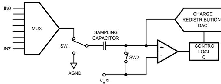
**Figure 4. ADC128S102 in Track Mode**
