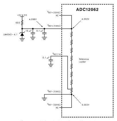
Figure 13. Using the V<sub>REF</sub> Force Pins Only
