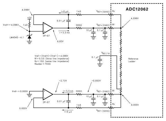
Figure 12. Reference Ladder Force and Sense Inputs
