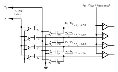
Figure 7. The Capacitive Voltage Divider
