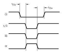
Figure 3.  $\overline{\text{CS}}$  Setup and Hold Timing for S/ $\overline{\text{H}}$ ,  $\overline{\text{RD}}$ , and OE
