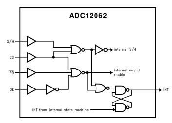
Figure 8. ADC Control Logic
