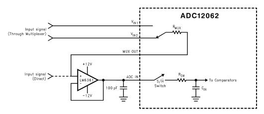
Figure 10. Buffering the Input with an LM6361 High Speed Op Amp
