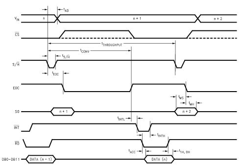
Figure 1. Interrupt Interface Timing (MODE = 1, OE = 1)
