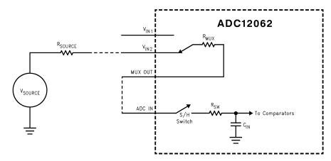
Figure 9. Simplified ADC12062 Input Stage
