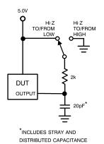
Figure 3. t<sub>EN</sub>, t<sub>DIS</sub> Test Circuit
