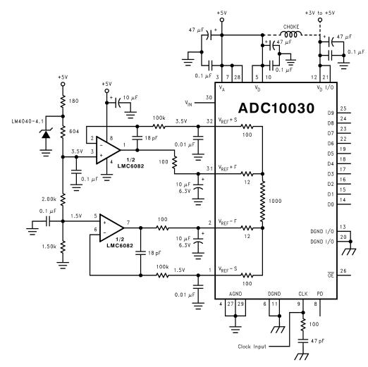
Figure 6. Setting Precision Reference Voltages
