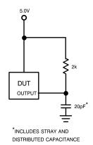
Figure 2. AC Test Circuit
