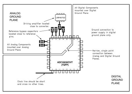
Figure 7. An Acceptable Layout Pattern for the ADC10030
