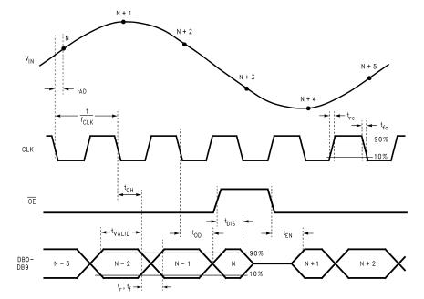
Figure 1. ADC10030 Timing Diagram
