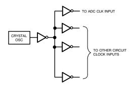
Figure 8. Isolating the ADC Clock from Digital Circuitry
