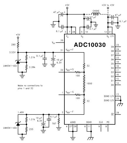
Figure 5. Improved Low Component Count Reference Biasing
