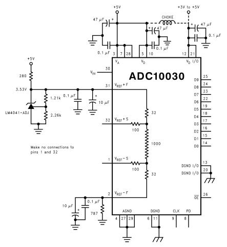
Figure 4. Simple, Low Component Count Reference Biasing
