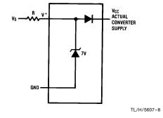
FIGURE 3. An On-Chip Shunt Regulator Diode
