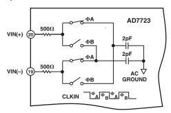
Figure 15. Analog Input Equivalent Circuit
