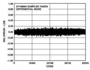
TPC 10. Differential Nonlinearity (Output Data Rate = 600 kHz)
