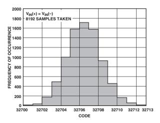
TPC 7. Histogram of Output Codes with DC Input (Output Data Rate = 1.2 MHz)
