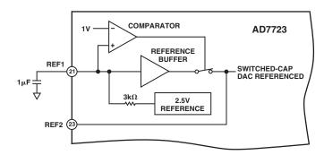
Figure 19. Reference Circuit Block Diagram
