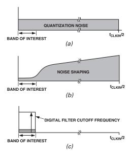
Figure 9. Sigma-Delta ADC
