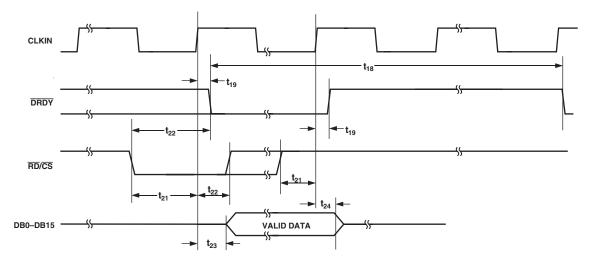
Figure 7b. Parallel Mode Read Timing,  $\overline{CS} = \overline{RD}$
