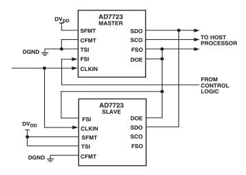
Figure 24. Serial Mode 1 Connection for Two-Channel Multiplexed Operation
