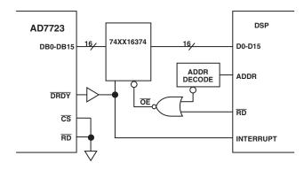
Figure 23. Parallel Interface Connection
