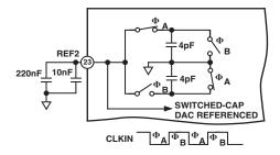
Figure 20. REF2 Equivalent Input Circuit
