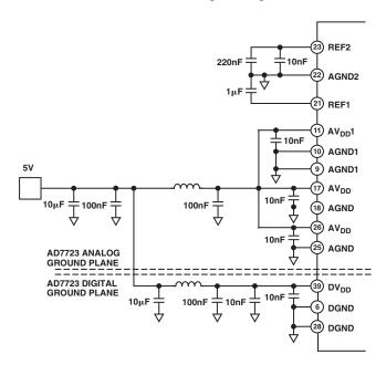
Figure 29. Reference and Power Supply Decoupling
