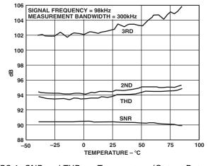
TPC 4. SNR and THD vs. Temperature (Output Data Rate = 600 kHz)
