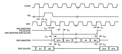
Figure 25. Serial Mode 1 Timing for Two-Channel Multiplexed Operation
