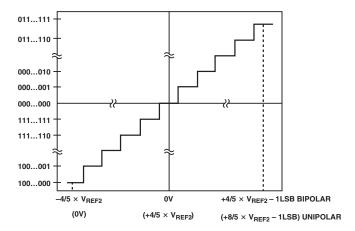
Figure 13. Bipolar (Unipolar) Mode Transfer Function
