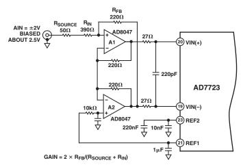
Figure 17. Single-Ended-to-Differential Input Circuit for Bipolar Mode Operation (Analog Input Biased About 2.5 V)
