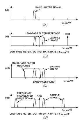
Figure 10. Band-Pass Operation
