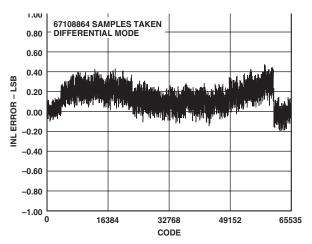
TPC 12. Integral Nonlinearity (Output Data Rate = 600 kHz)
