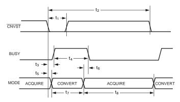
Figure 11. Basic Conversion Timing
