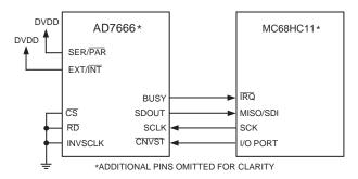
Figure 21. Interfacing the AD7666 to SPI Interface
