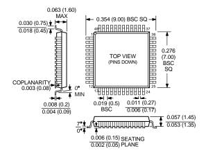
48-Lead Frame Chip Scale Package (LQFP) (CP-48)
