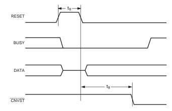
Figure 12. RESETTiming
