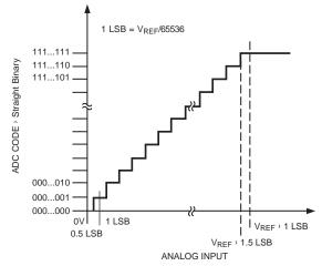
Figure 4. ADC Ideal Transfer Function
