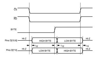
Figure TBD, 8-bit Parallel Interface
