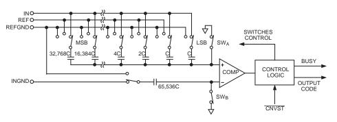
Figure 3. ADC Simplified Schematic
