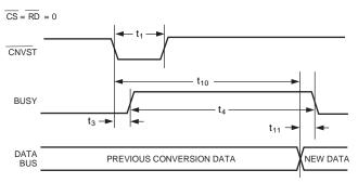
Figure 13. Master Parallel Data Timing for Reading (Continuous Read)
