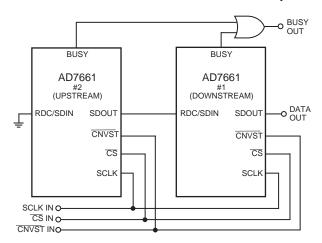
Figure 19. Two AD7661s in a "Daisy-Chain" Configuration
