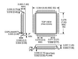
48-Lead Frame Chip Scale Package (LQFP) (CP-48)
