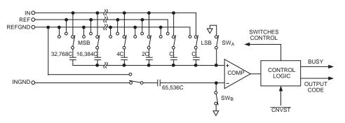
Figure 3. ADC Simplified Schematic
