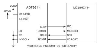
Figure 21. Interfacing the AD7661 to SPI Interface
