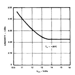
Linearity vs. Power Supply Voltage
