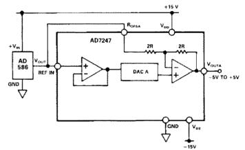
Figure 9. Bipolar Configuration
