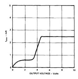
Single Supply Sink Current vs. Output Voltage
