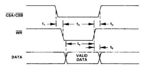
Figure 5. AD7247 Write Cycle Timing Diagram
