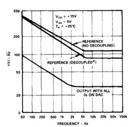
\*REFERENCE DECOUPLING COMPONENTS ARE a 200  $\Omega$  RESISTOR IN SERIES WITH A PARALLEL COMBINATION OF 10  $\mu F$  AND 0.1  $\mu F$  TO GND.
