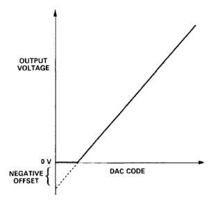
Figure 1. Effect of Negative Offset (Single Supply)
