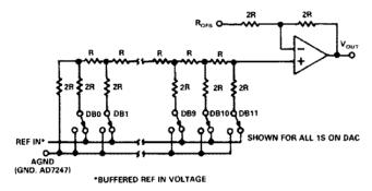
Figure 2. D/A Simplified Circuit Diagram
