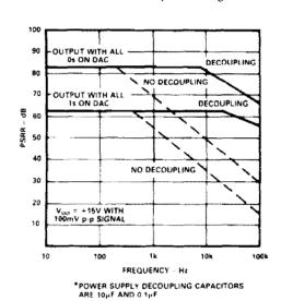
Power Supply Rejection Ratio vs. Frequency
