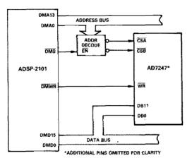
Figure 10. AD7247 to ADSP-2101 Interface
