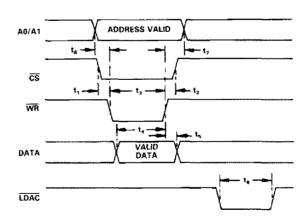
Figure 7. AD7237 Write Cycle Timing Diagram
