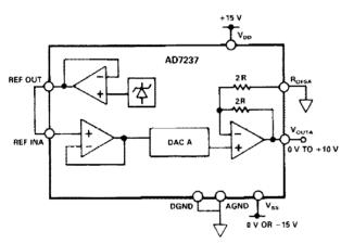
Figure 8. Unipolar (0 to +10 V) Configuration
