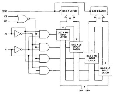
Figure 6. AD7237 Input Control Logic
