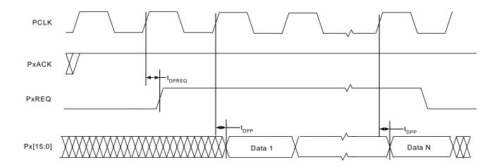
Figure 14. Slave Mode PxREQ to PCLK Switching Characteristics
