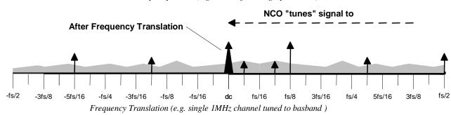
Figure 28. AD6652 Frequency Translation of Wideband Input Spectrum
