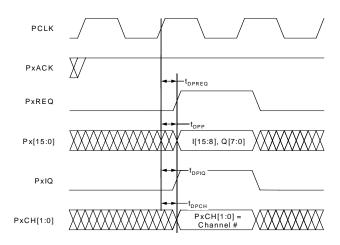
Figure 36. Channel mode 8I/8Q parallel format.
