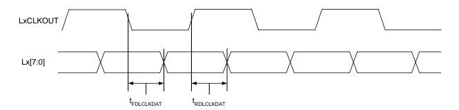
Figure 17. LxCLKOUT to Lx[7:0]Data Switching Characteristics
