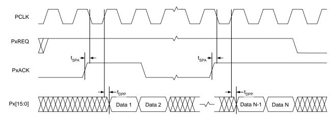
Figure 13. Slave Mode PxACK to PCLK Switching Characteristics
