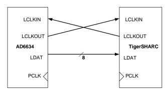
Figure 39. Link Port Connection Between AD6652 and TigerSHARC
