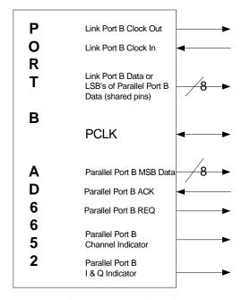
Figure 34. Output Port Configuration
