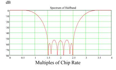
Figure 31. Interpolating Halfband Frequency Response
