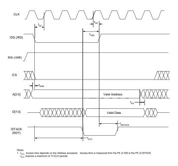
Figure 21. MNM Microport Read Timing Requirements.
