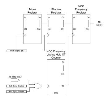
Figure 33. NCO Shadow Register and Hold Off Counter
