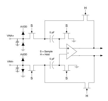
Figure 22. Switched-Capacitor SHA Input for one ADC channel
