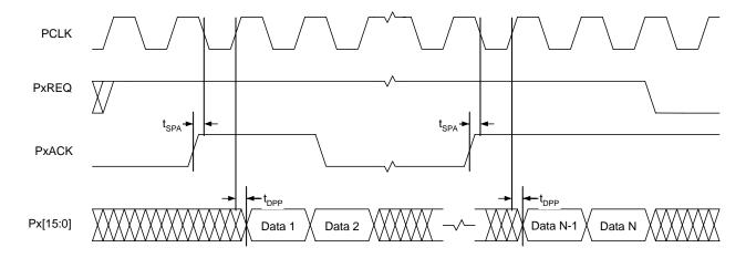
Figure 10. Master Mode PxACK to PCLK Switching Characteristics
