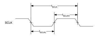
Figure 43. SCLK Timing Requirements
