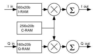
Figure 30. RAM Coefficient Filter Block Diagram
