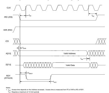
Figure 19. INM Microport Read Timing Requirements.
