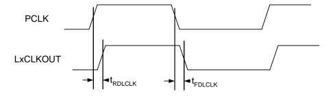
Figure 15. LxCLKOUT to PCLK Switching Characteristics
