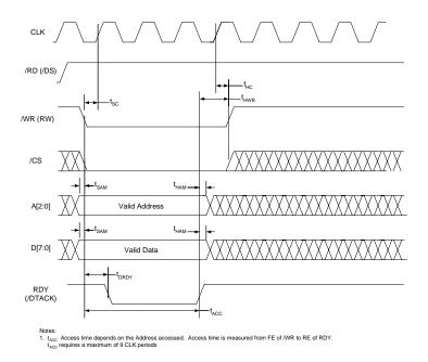
Figure 18. INM Microport Write Timing Requirements.
