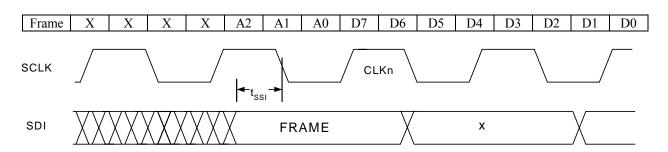
Figure 46. Serial Word Structure and Serial Port Control Timing
