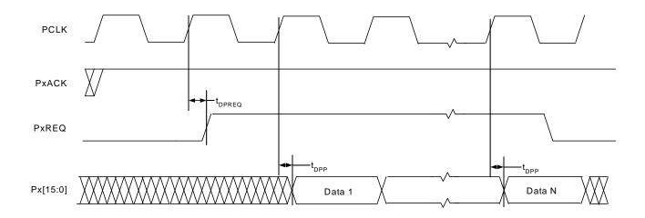
Figure 11. Master Mode PxREQ to PCLK Switching Characteristics
