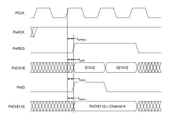
Figure 35. Channel mode interleaved format.
