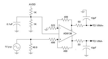
Figure 23. Differential Input for a single channel of the AD6652 using the AD8138 for Nyquist applications (dc to 32.5 MHz).
