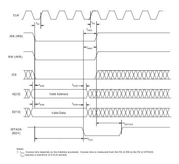
Figure 20. MNM Microport Write Timing Requirements.
