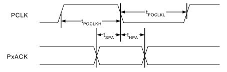
Figure 12. Slave Mode PxACK to PCLK Setup and Hold Characteristics
