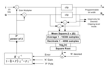
Figure 32: Block Diagram of the AGC
