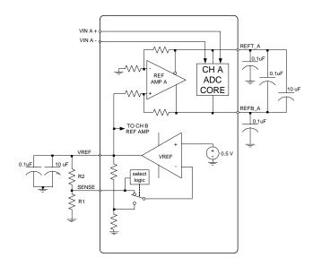
Figure 27. Programmable reference configuration showing the common VREF and Ch. A connections. Ch. B connections are identical to those of Ch. A.
